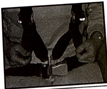
Pull Strap Ends To Tighten 190/195 & Luscombe
